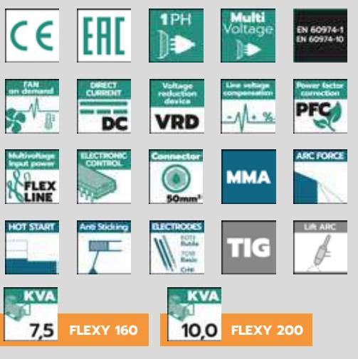
**EN** • MMA/TIG inverters technology machines designed to be powered from any input voltage between 90 to 270V. Thanks to the FLEX-LINE function, the device automatically recognizes the value of the input power supply (110V or 220V). Equipped with the PFC function, which ensures high efficiency of the units and allows to weld with high currents and low consumptions.
