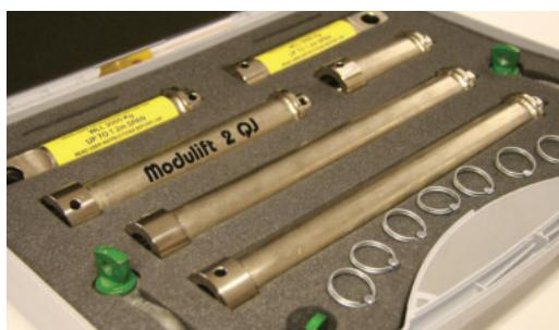
The Modulift spreader is modular in length and every spreader consists of 1 pair of End Units and Drop Links, with intermediate struts that can be bolted into the assembly to achieve different spans. The MOD 6 has an assembled span ranging from 400 mm to 4,5 m in 100 mm increments.
